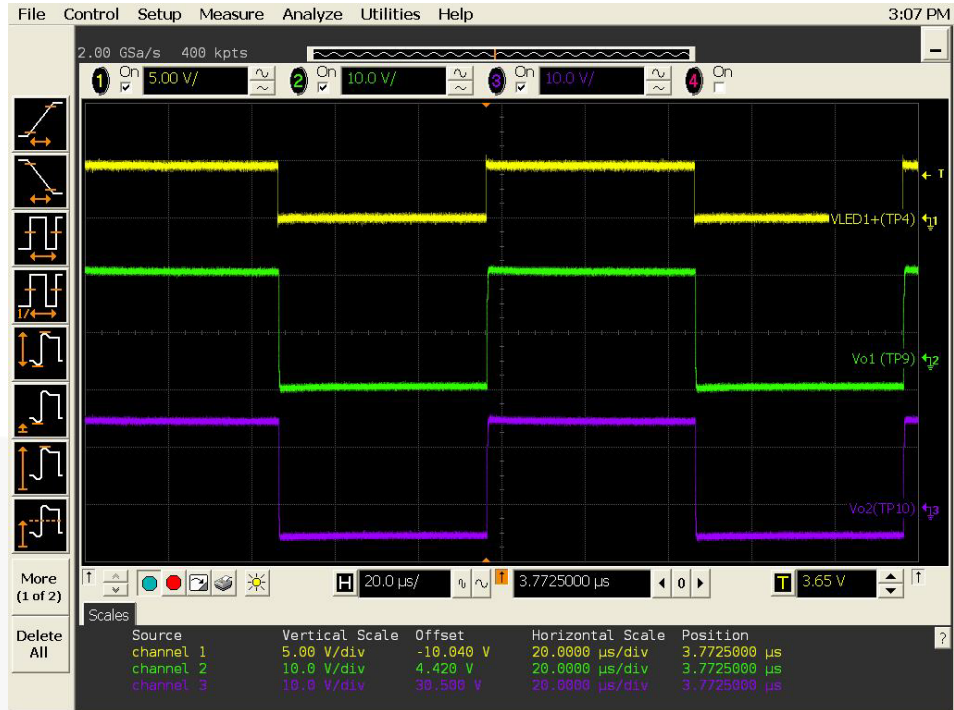
Figure 9. FOD833x with Totem-Pole Current Buffer - V_{LED1+} , V_{O1} and V_{O2} Waveform
