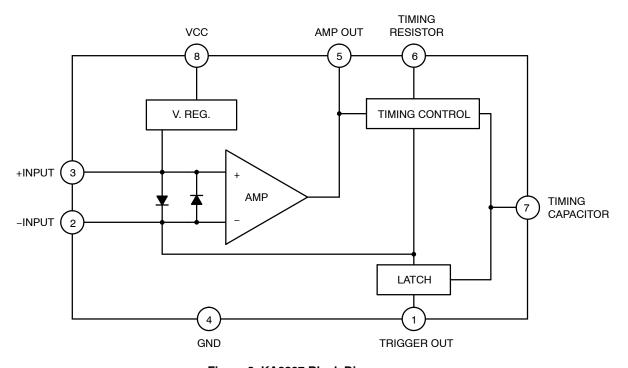
Figure 2. KA2807 Block Diagram
