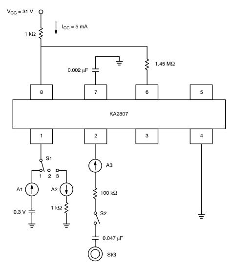
Figure 3. KA2807 Test Circuit
