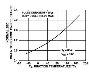
Figure 12. Normalized R<sub>DSON</sub> vs. Junction Temperature
