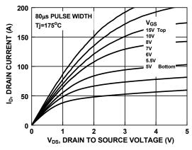
Figure 10. Saturation Characteristics
