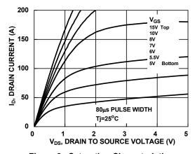
Figure 9. Saturation Characteristics
