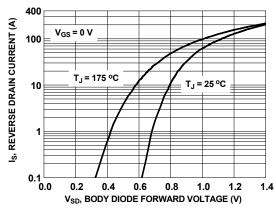
Figure 8. Forward Diode Characteristics
