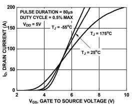
Figure 7. Transfer Characteristics
