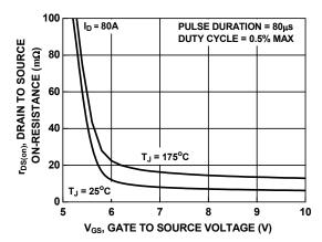
Figure 11. R<sub>DSON</sub> vs. Gate Voltage
