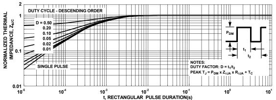
Figure 3. Normalized Maximum Transient Thermal Impedance
