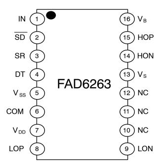
Figure 3. Pin Connection (Top View)
