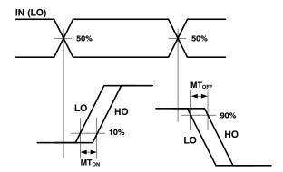
Figure 34. Delay Matching Waveform Definition
