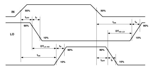
Figure 33. Switching Time and Dead-Time Waveform Definition
