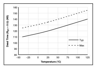
Figure 8. Dead Time ( $R_{DT}$  = 0  $\Omega$ ) vs. Temperature
