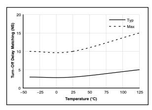
Figure 13. Turn-Off Delay Matching vs. Temperature
