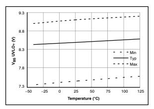
Figure 21.  $V_{BS}$  UVLO+ vs. Temperature
