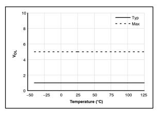
Figure 24. Low-Level Output Voltage vs. Temperature
