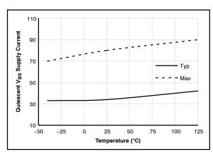
Figure 17. Quiescent V<sub>BS</sub> Supply Current vs. Temperature
