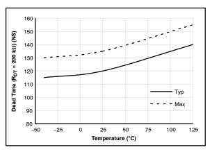
Figure 10. Dead Time (R<sub>DT</sub> = 200 k $\Omega$ ) vs. Temperature
