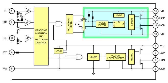
Figure 2. Simplified Block Diagram
