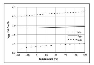
Figure 20. V<sub>DD</sub> UVLO- vs. Temperature
