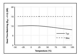
Figure 9. Dead Time Matching ( $R_{DT}$  = 0  $\Omega$ ) vs. Temperature
