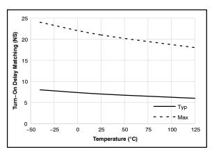
Figure 12. Turn-On Delay Matching vs. Temperature
