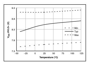
Figure 19.  $V_{DD}$  UVLO+ vs. Temperature
