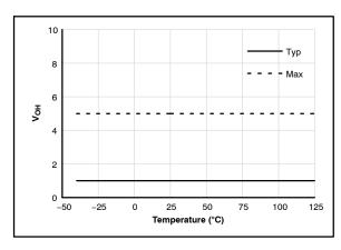
Figure 23. High-Level Output Voltage vs. Temperature
