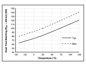
Figure 11. Dead Time Matching ( $R_{DT}$  = 200 k $\Omega$ ) vs. Temperature
