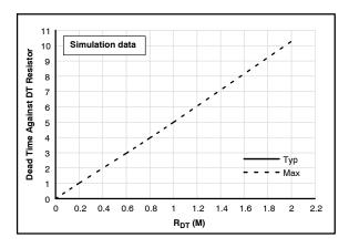
Figure 14. Dead Time vs. R<sub>DT</sub>
