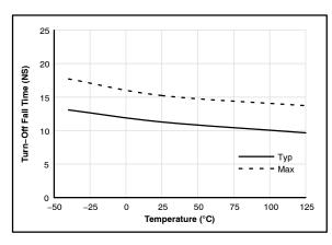
Figure 7. Turn-Off Fall Time vs. Temperature
