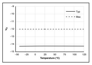
Figure 28. Allowable Negative  $V_{\mbox{\scriptsize S}}$  Voltage vs. Temperature
