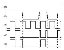
Figure 37. Shutdown with SR Pin Pulled Down SR Pin Pulled Up
