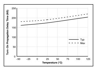
Figure 4. Turn-On Propagation Delay vs. Temperature
