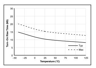
Figure 6. Turn-On Rise Time vs. Temperature
