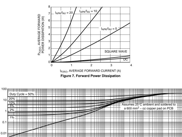
PULSE TIME (sec) **Figure 8. Thermal Response**
