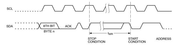
Figure 3. Write Cycle Timing
