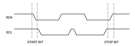
Figure 4. Start/Stop Timing
