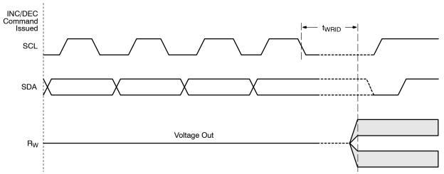
Figure 13. Increment/Decrement Timing Limits
