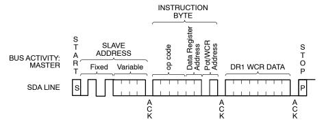
Figure 7. Write Timing
