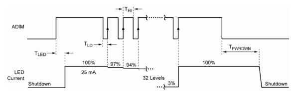
Figure 28. ADIM Dimming Timing Diagram (no C<sub>PWM</sub>, PWM high)
