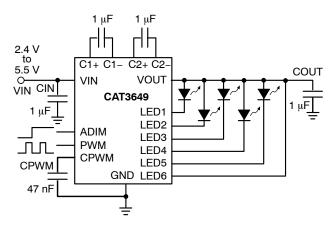
Figure 30. Application with 5 LEDs
