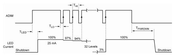
Figure 2. ADIM Dimming Timing Diagram (no C<sub>PWM</sub>, PWM high)
