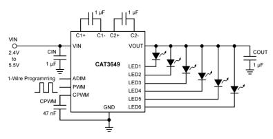
Figure 1. Typical Application Circuit
