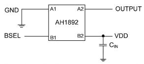
Note: C<sub>IN</sub> is for power stabilization and to strengthen the noise immunity, the recommended capacitance is 100nF typical
