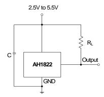
Note: 5. C is for power stabilization and to strengthen the noise immunity, the recommended capacitance is 10nF to 100nF.  $R_L$  is the pull-up resistor, the recommended resistance is 10k $\Omega$  to 100k $\Omega$ .
