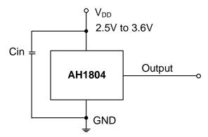
Note: Cin is for power stabilization and to strengthen the noise immunity, C = 100nF or higher must be used.
