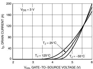
Figure 2. Transfer Characteristics
