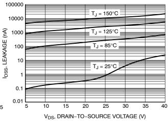
Figure 6. Drain-to-Source Leakage Current vs. Voltage
