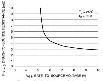
Figure 3. On-Resistance vs. Gate-to-Source Voltage
