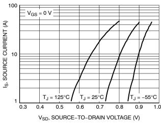
Figure 10. Diode Forward Voltage vs. Current
