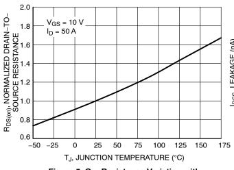
Figure 5. On–Resistance Variation with Temperature
