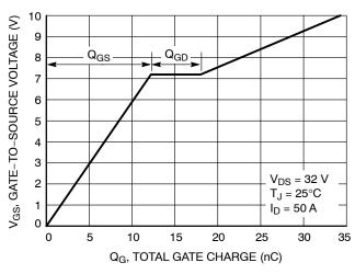
Figure 8. Gate-to-Source vs. Total Charge
