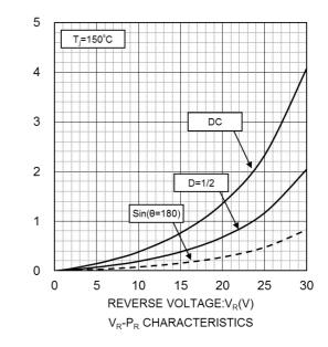
REVERSE POWER DISSIPATION:P<sub>R</sub>(W)
