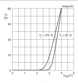
$V_{DS} > I_D \times R_{DSon}$
