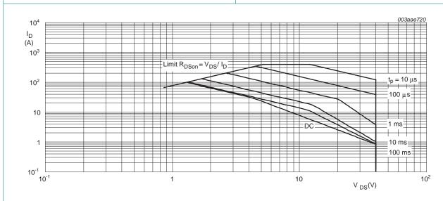
$T_{mh} = 25$  °C;  $I_{DM}$  is a single pulse
