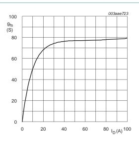
$T_j = 25 \,^{\circ}\text{C}; \ V_{DS} = 15 \,^{\circ}\text{V}$
