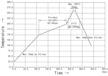
Recommended lead free reflow soldering temperature profile.
