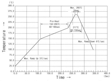
Recommended lead free reflow soldering temperature profile.
