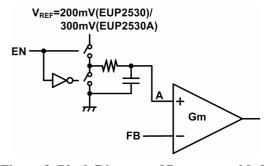
Figure 3. Block Diagram of Programmable FB Voltage Using PWM Signal
