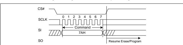
Figure31. Program/Erase Resume Sequence Diagram
