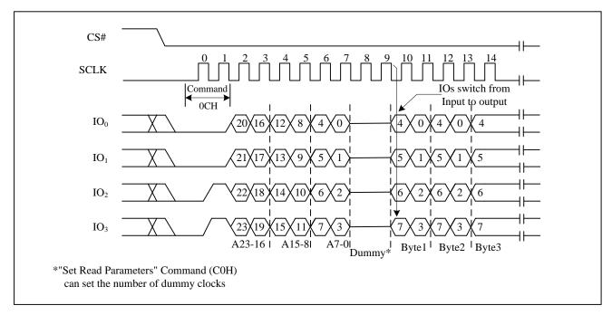
Figure37. Burst Read with Wrap command Sequence Diagram
