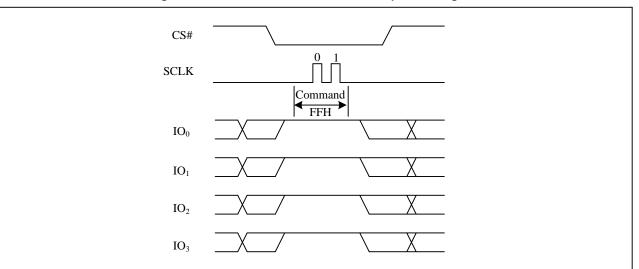
Figure 41. Disable QPI mode command Sequence Diagram
