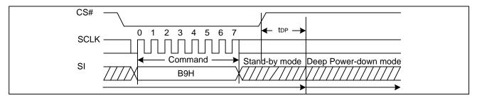
Figure23a. Deep Power-Down Sequence Diagram (QPI)
