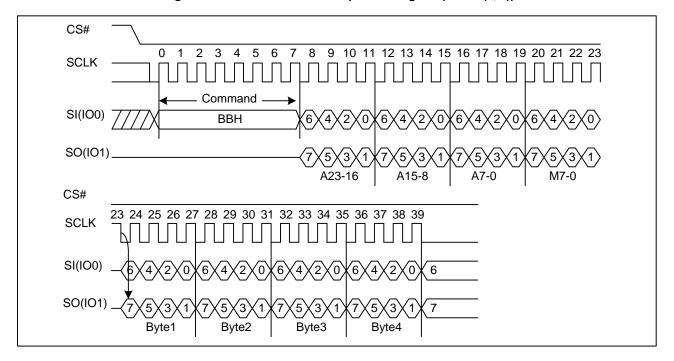
Figure13. Dual I/O Fast Read Sequence Diagram (M5-4≠ (1, 0))
