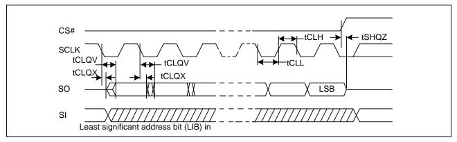
Figure49. Resume to Suspend Timing Diagram
