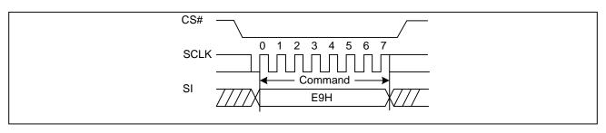
Figure3a. Disable 4-byte Mode Sequence Diagram (QPI)
