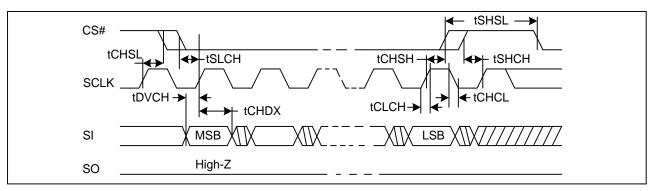
Figure48. Output Timing
