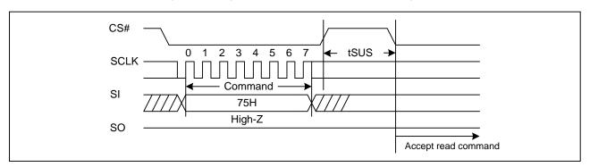
Figure 30. Program/Erase Suspend Sequence Diagram
