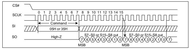
Figure7a. Read Status Register Sequence Diagram (QPI)
