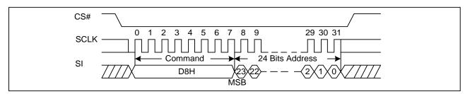
Figure 21. 64KB Block Erase Sequence Diagram
