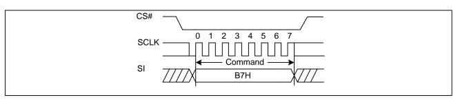
Figure2a. Enable 4-byte Mode Sequence Diagram (QPI)
