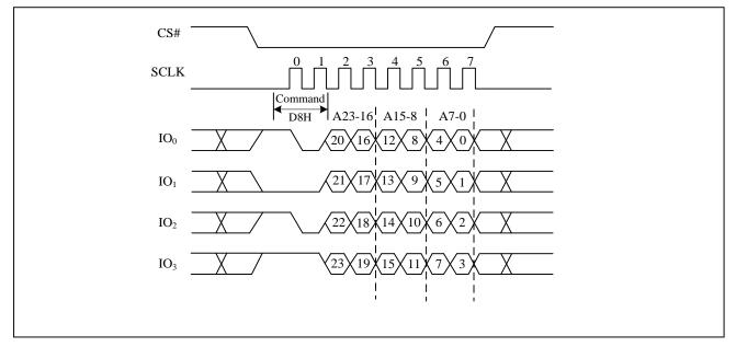
Figure21a. 64KB Block Erase Sequence Diagram (QPI)
