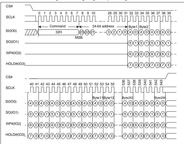
Figure18.Quad Page Program Sequence Diagram
