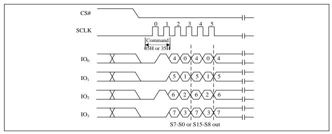
Figure7b. Read Status Register Sequence Diagram (QPI) (15H)
