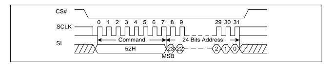
Figure20. 32KB Block Erase Sequence Diagram
