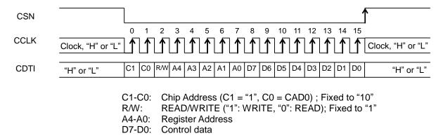
Figure 41. Serial Control I/F Timing (CSP pin = "L")
