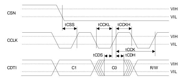
Figure 13. WRITE Command Input Timing (CSP pin = "L")
