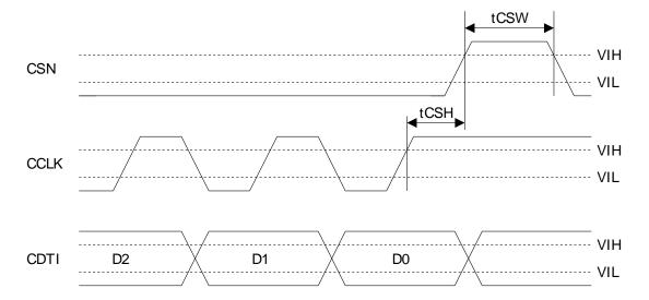
Figure 14. WRITE Data Input Timing (CSP pin = "L")
