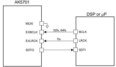
Figure 21. PLL Slave Mode 2 (PLL Reference Clock: EXLRCK or EXBCLK pin)
