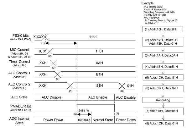
Figure 52. MIC Input Recording Sequence
