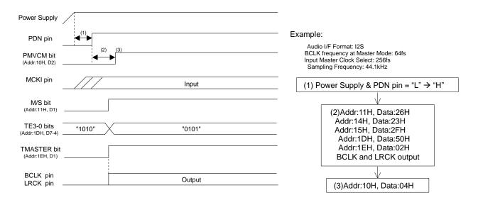
Figure 49. Clock Set Up Sequence (5)
