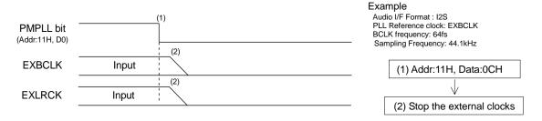
Figure 54. Clock Stopping Sequence (2)
