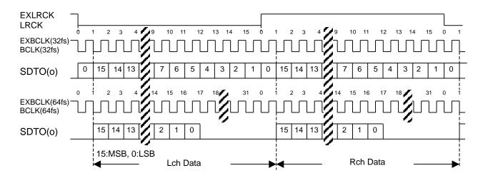
Figure 35. Mode 3 Timing ( $I^2S$ , M/S = "0" or "1")
