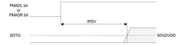
Figure 17. Power Down & Reset Timing 1
