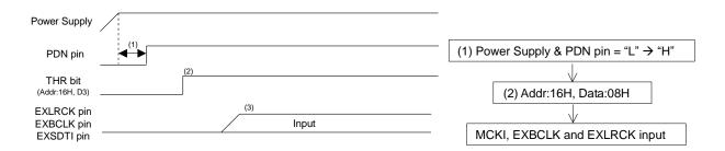
Figure 51. Clock Set Up Sequence (7)
