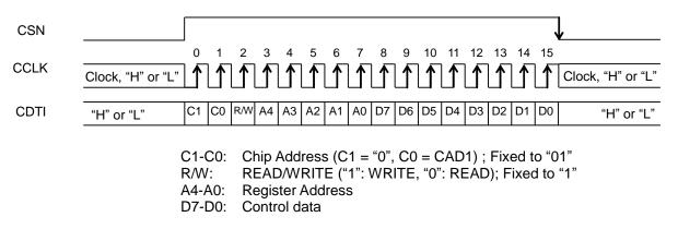
Figure 42. Serial Control I/F Timing (CSP pin = "H")
