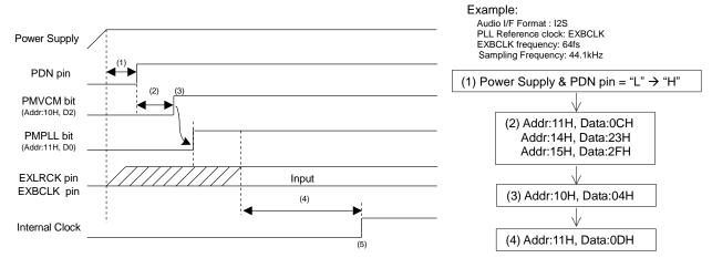
Figure 46. Clock Set Up Sequence (2)
