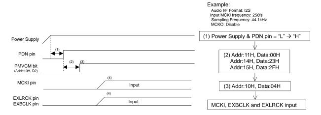
Figure 48. Clock Set Up Sequence (4)
