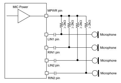
Figure 38. MIC Block Circuit
