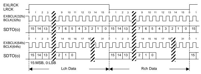
Figure 34. Mode 2 Timing (MSB justified, M/S = "0" or "1")
