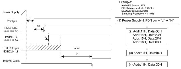
Figure 50. Clock Set Up Sequence (6)
