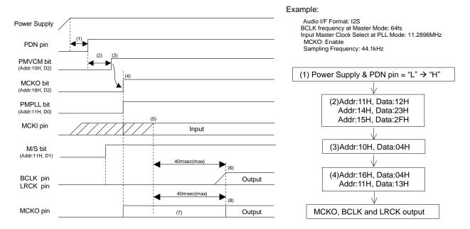
Figure 45. Clock Set Up Sequence (1)
