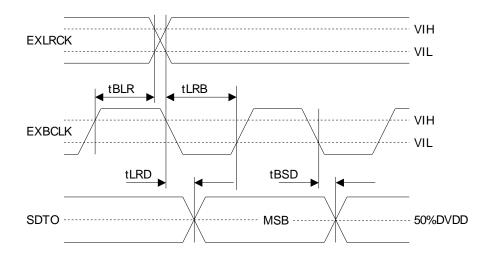
Figure 12. Audio Interface Timing (PLL/EXT Slave mode)
