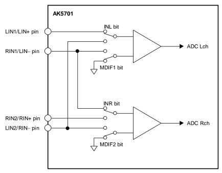
Figure 36. Mic/Line Input Selector
