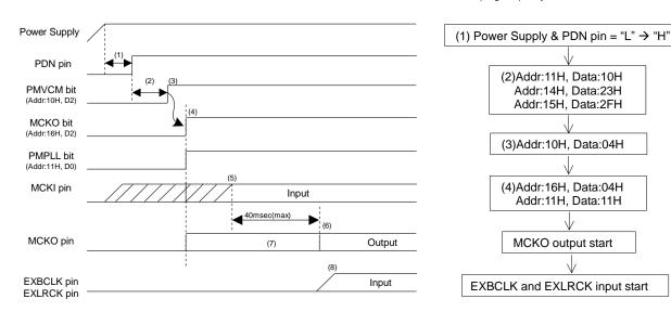
Figure 47. Clock Set Up Sequence (3)
