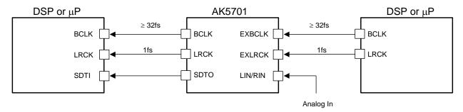
Figure 25. Slave & Bypass Mode
