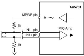
Figure 37. Connection Example for Full-differential Mic Input (MDIF1/2 bits = "1")
