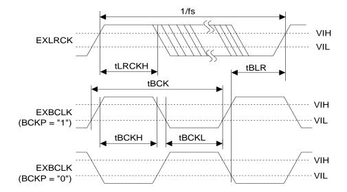
Figure 7. Clock Timing (PLL Slave mode; PLL Reference Clock = EXLRCK or EXBCLK pin & DSP mode; MSBS = 1)
