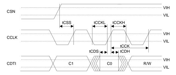
Figure 15. WRITE Command Input Timing (CSP pin = "H")
