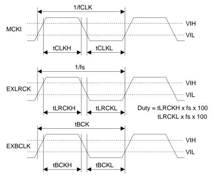
Figure 11. Clock Timing (EXT Slave mode)
