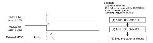
Figure 55. Clock Stopping Sequence (3)
