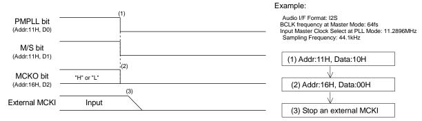
Figure 53. Clock Stopping Sequence (1)
