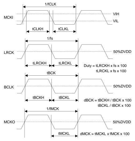
Figure 2. Clock Timing (PLL/EXT Master mode)
