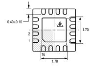
For reference only, not for tooling use (reference JEDEC MO-220WEED) Dimensions in millimeters
