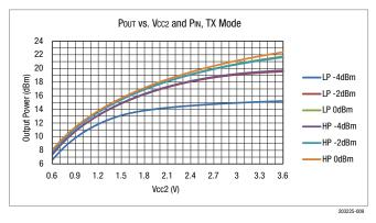
Figure 9. Pout vs. Vcc2 and PiN (Vcc1 = 1.8 V, Vdd = 3.0 V, f = 2440 MHz)
