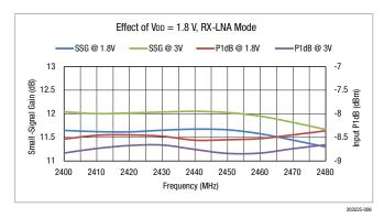
Figure 6. Effect of Lowering VDD (VCC1 = VCC2 = 1.8 V, PIN = -25 dBm, RX-LNA Mode)
