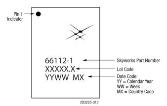
Figure 13. SKY66112-11 Typical Part Marking (Top View)
