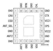
Figure 2. SKY66112-11 Pinout (Top View)
