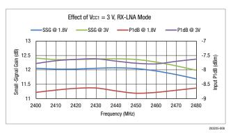
Figure 8. Effect of Raising Vcc1 (Vcc2 = VDD = 3.0 V, PIN = -25 dBm, RX-LNA Mode)
