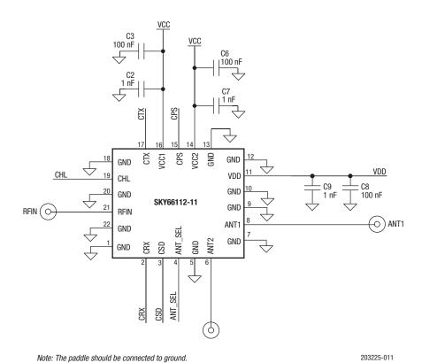
Figure 11. SKY66112-11 Reference Design Schematic
