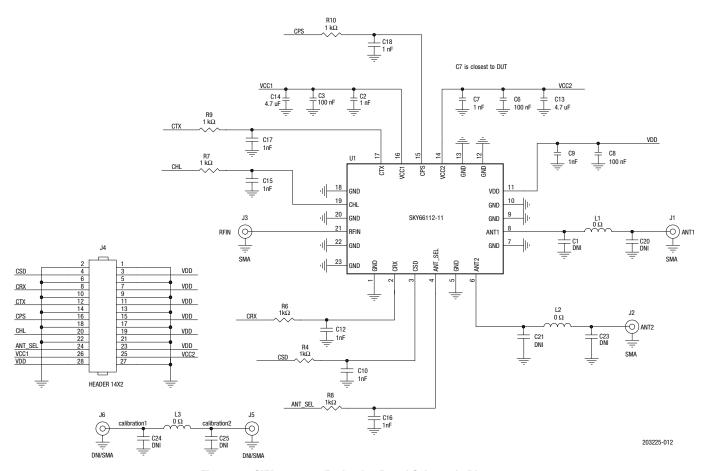
Figure 12. SKY66112-11 Evaluation Board Schematic Diagram
