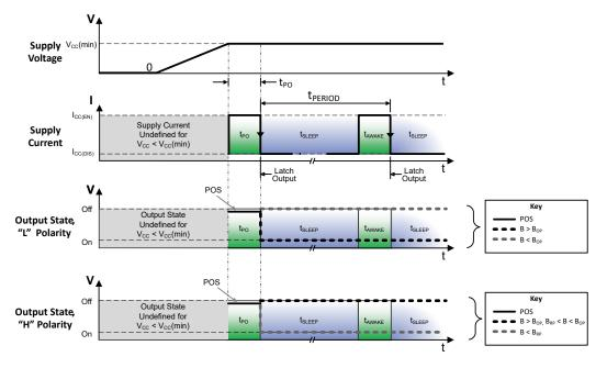
Figure 4: Micropower Operation and Power-On Behavior
