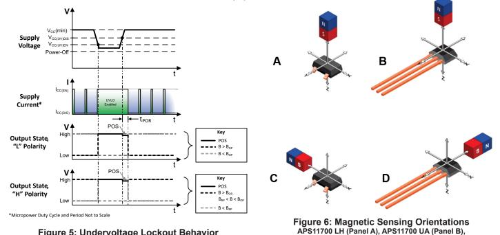
Figure 5: Undervoltage Lockout Behavior
