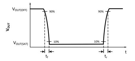
Figure 2: Definition of Output Rise and Fall Time
