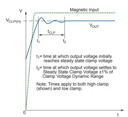
Figure 2: Delay to Clamp Definition
