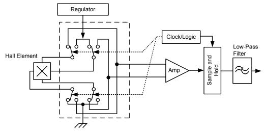
**Concept of Chopper Stabilization Technique**
