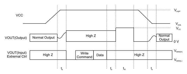
Figure 15: Write to Non-Volatile Memory (EEPROM)
