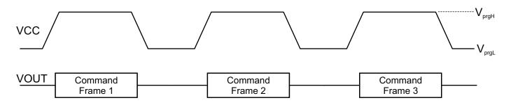
Figure 12: Format for Sending Multiple Transactions
