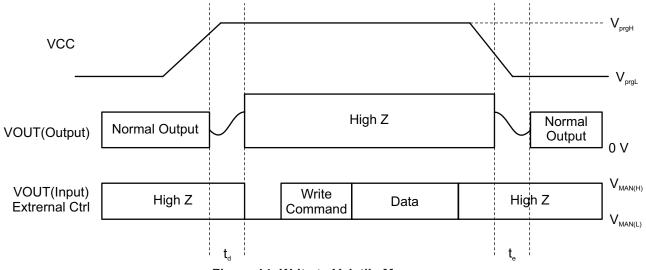
Figure 14: Write to Volatile Memory
