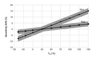
Figure 6: Sensitivity Drift Through Temperature Range (ΔSensTC)
