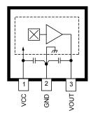
**UC Package Pinout Diagram**
