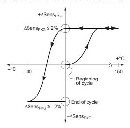
Figure 7: Package Hysteresis Sensitivity Drift
