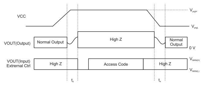
Figure 13: Write Access Code
