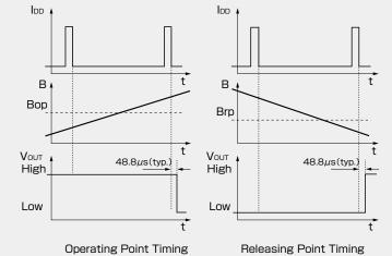
This Hall effect IC's output is held as internal data just before the internal circuit 38 turns OFF (IDD OFF). And after 48.8  $\,\mu$  s, the output changes.
