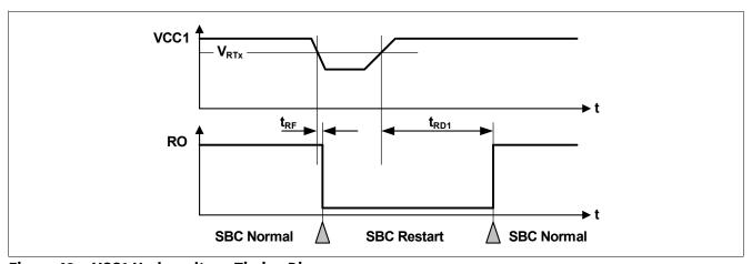
Figure 43 VCC1 Undervoltage Timing Diagram
