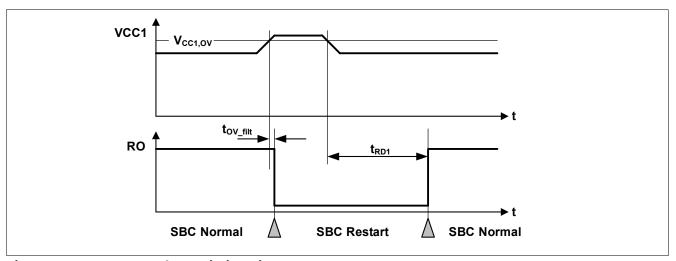
Figure 44 VCC1 Overvoltage Timing Diagram
