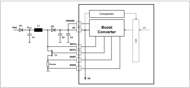
Figure 9 Boost Block Diagram
