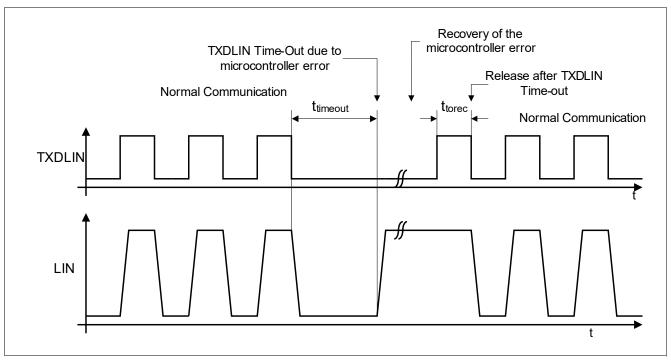
Figure 26 TXDLIN Time-Out Function
