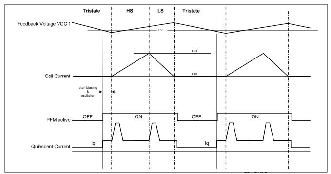
Figure 8 Typical PFM timing diagram
