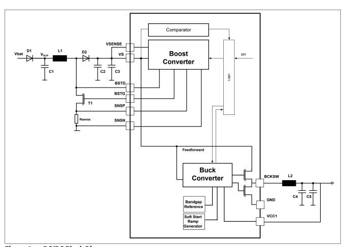
Figure 6 DC/DC Block Diagram
