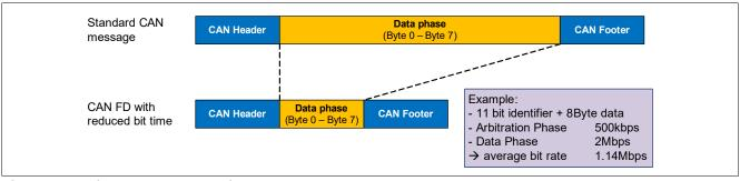
Figure 18 Bite rate Increase with CAN FD vs. Standard CAN
