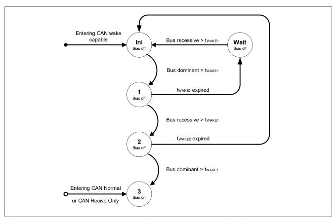
Figure 20 CAN Wake-up Pattern Detection (WUP) according to the Definition in ISO 11898-5
