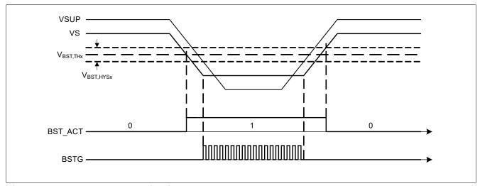
Figure 10 Boost converter activation
