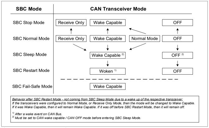
Figure 17 CAN Mode Control Diagram
