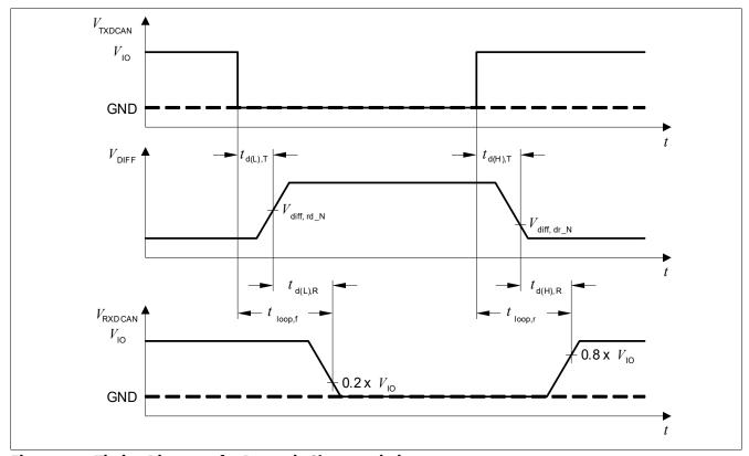
Figure 21 Timing Diagrams for Dynamic Characteristics
