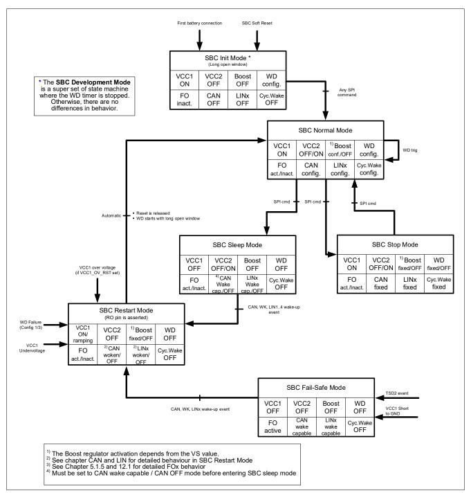
Figure 3 State diagram showing the SBC operating modes
