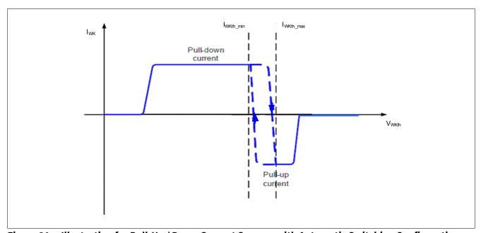
Figure 31 Illustration for Pull-Up / Down Current Sources with Automatic Switching Configuration
