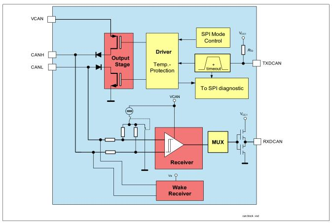
Figure 16 Functional Block Diagram
