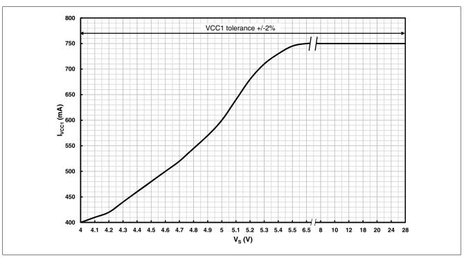
Figure 12 Maximum DCDC Buck current capability versus VS.
