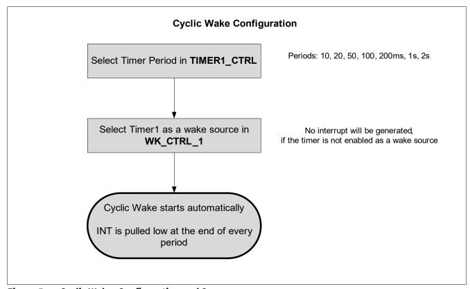
Figure 5 Cyclic Wake: Configuration and Sequence
