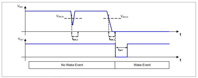
Figure 30 Wake-up Filter Timing for Static Sense
