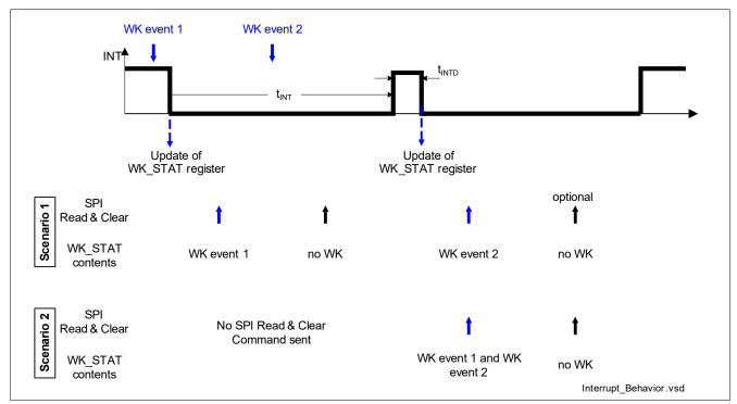
Figure 33 Interrupt Signaling Behavior
