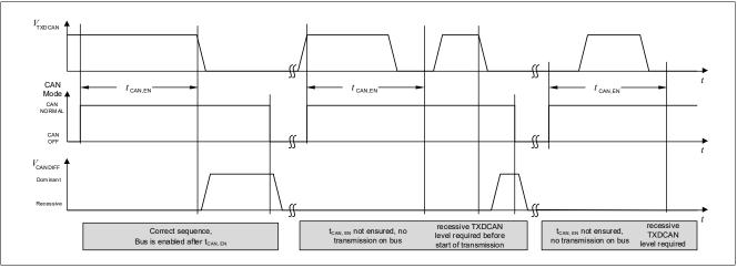
Figure 19 CAN Transceiver Enabling Sequence
