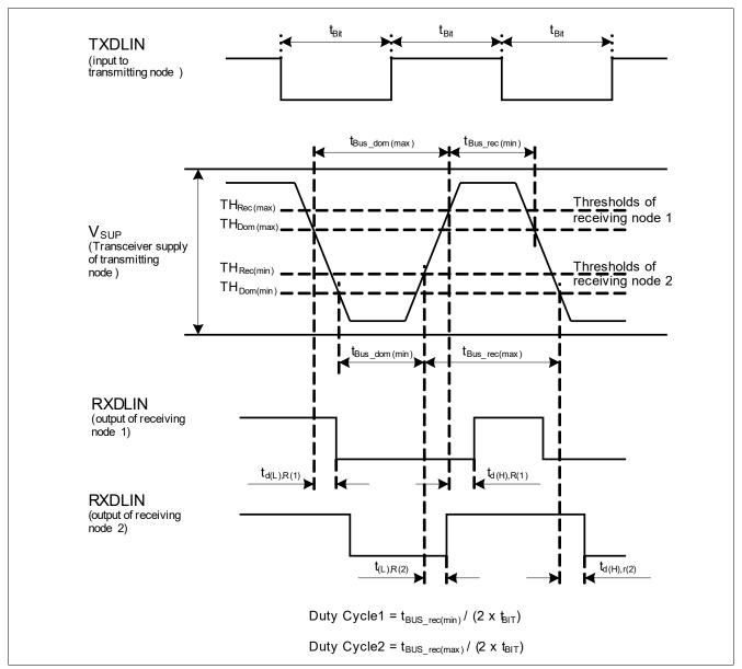
Figure 28 Timing Diagram for Dynamic Characteristics
