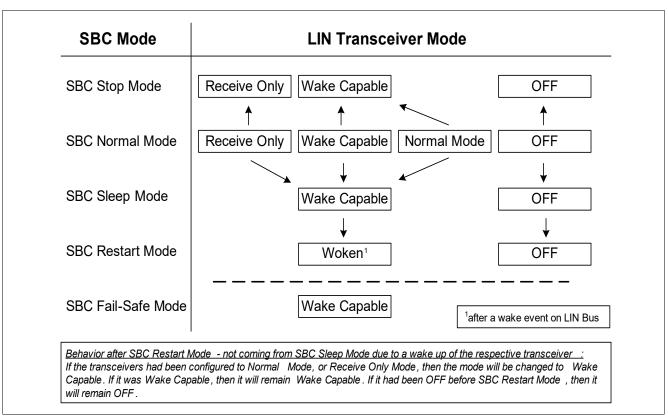
Figure 24 LIN Mode Control Diagram
