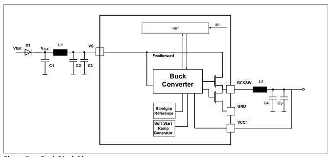
Figure 7 Buck Block Diagram
