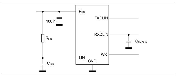
Figure 27 Simplified Test Circuit for Dynamic Characteristics
