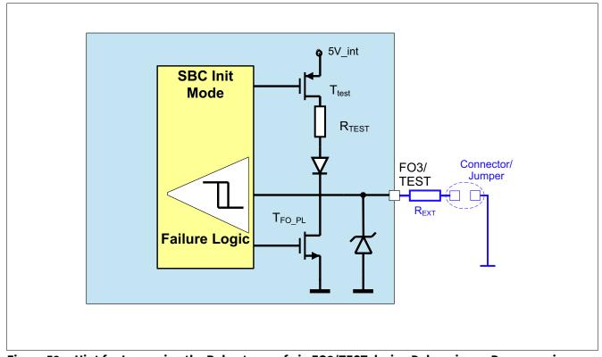
Figure 52 Hint for Increasing the Robustness of pin FO3/TEST during Debugging or Programming
