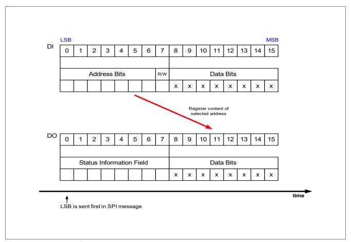
Figure 46 SPI Operation Mode
