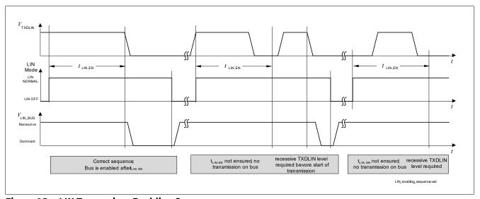
Figure 25 LIN Transceiver Enabling Sequence
