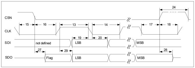
Figure 49 **SPI Timing Diagram**
