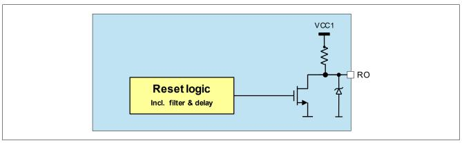
Figure 36 Reset Block Diagram
