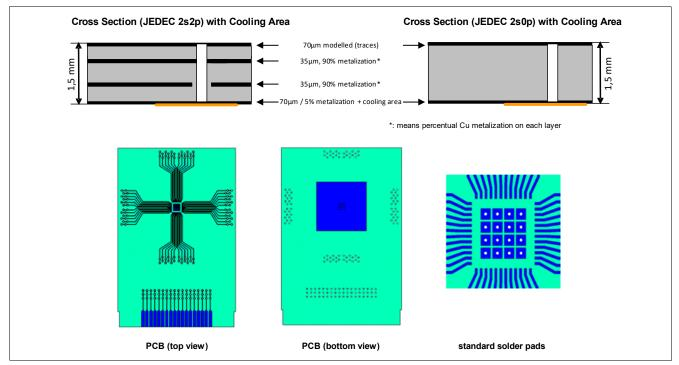
Figure 54 Board Setup
