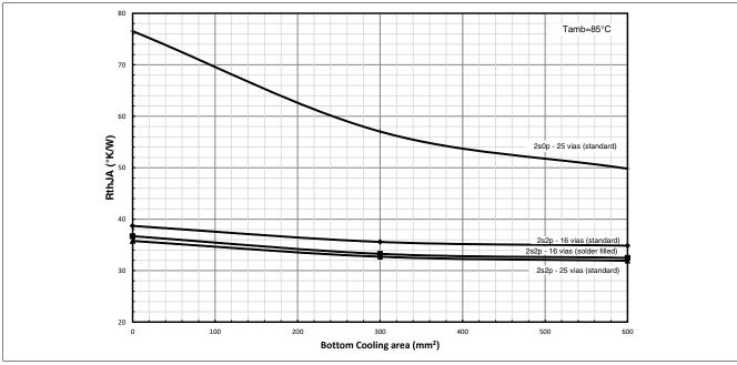
Figure 53 Thermal Resistance (Rth\_JA) vs. Cooling Area
