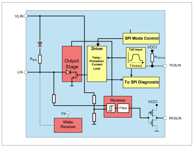
Figure 23 Block Diagram
