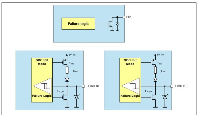
Figure 34 Fail-Safe Input and Outputs Block Diagrams
