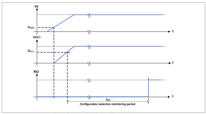
Figure 4 Hardware Configuration Selection Timing Diagram
