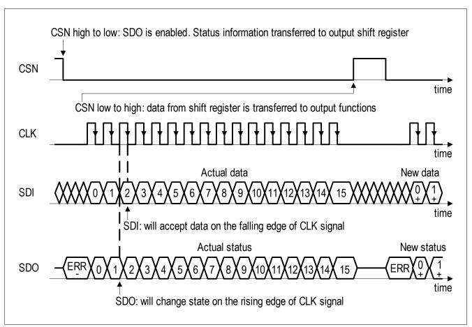
Figure 45 SPI Data Transfer Timing (note the reversed order of LSB and MSB shown in this figure compared to the register description)
