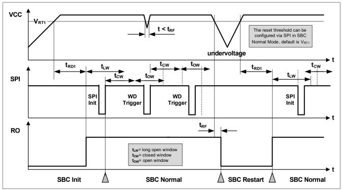
Figure 37 Reset timing Diagram
