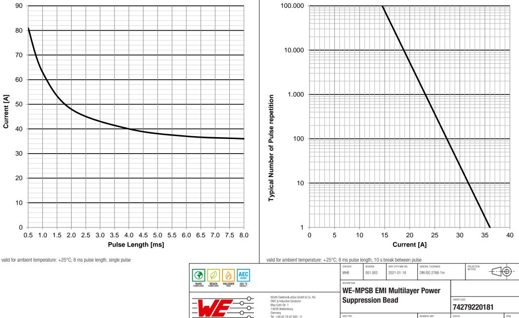
Typical Peak Current vs. Pulse Length Characteristics: Typical Number of Pulse Repetition:
