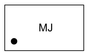
Note: The marking codes can be rotated by 90 ° or 180° to differentiate assembly location. In no case should this product marking be used to orient the component for its placement on a PCB. Only pin 1 mark is to be used for this purpose.
