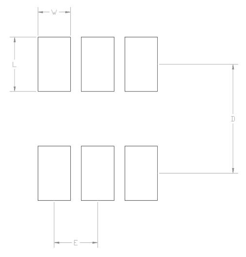
Figure 8.1. Si51210 6-pin TDFN PCB Land Pattern
