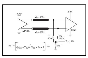
Figure 4A. 3.3V LVPECL Output Termination
