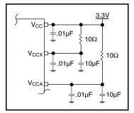
Figure 1. Power Supply Filtering
