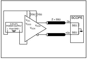
3.3V LVDS Output Load Test Circuit
