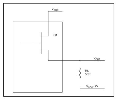
Figure 8. LVPECL Driver Circuit and Termination
