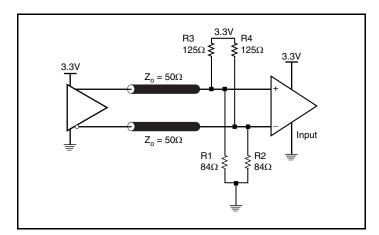
Figure 4B. 3.3V LVPECL Output Termination
