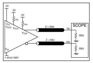
3.3V LVPECL Output Load Test Circuit
