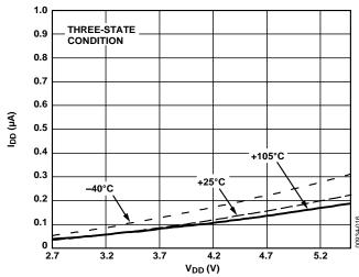
Figure 16. Power-Down Current vs. Supply Voltage
