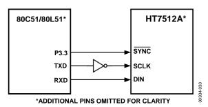
Figure 30. HT7512A to 80C51/80L51 Interface
