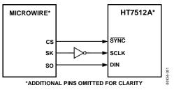
Figure 31. HT7512A to MICROWIRE Interface
