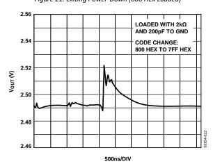
Figure 22. Digital-to-Analog Glitch Impulse
