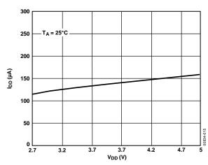
Figure 15. Supply Current vs. Supply Voltage
