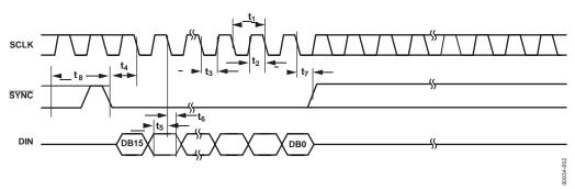
Figure 2. Serial Write Operation
