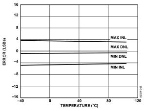
Figure 8. INL Error and DNL Error vs. Temperature
