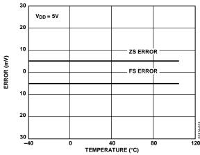
Figure 9. Zero-Scale Error and Full-Scale Error vs. Temperature
