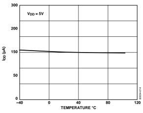
Figure 14. Supply Current vs. Temperature
