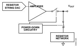
Figure 27. Output Stage During Power-Down
