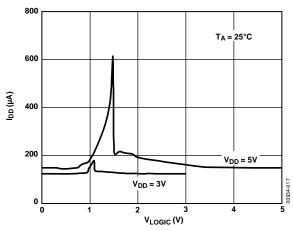
Figure 17. Supply Current vs. Logic Input Voltage
