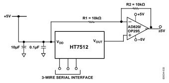
Figure 33. Bipolar Operation with the HT7512A
