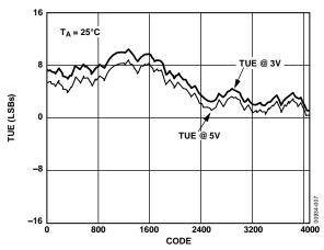
Figure 7. Typical Total Unadjusted Error Plot
