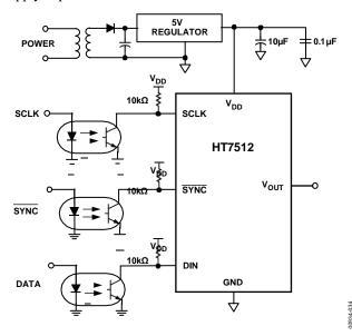
Figure 34. HT7512A with An Opto-Isolated Interface
