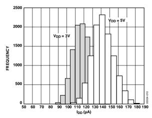
Figure 10.  $I_{DD}$  Histogram with  $V_{DD}$  = 3 V and  $V_{DD}$  = 5 V
