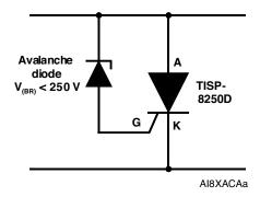
Figure 2. Overvoltage Protection Circuit
