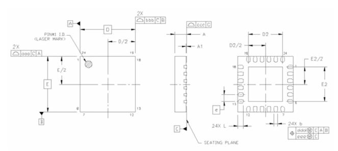
Figure 4. 24-Lead Quad Flat No-lead (QFN)
