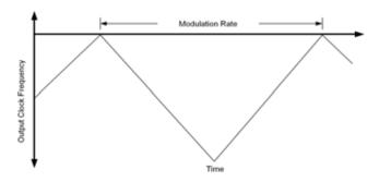
Figure 3. Spread Spectrum Triangle Waveform
