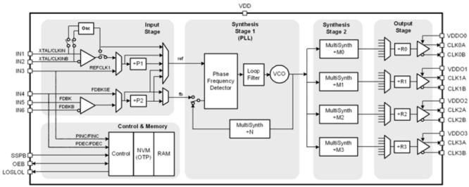
Figure 1. Si5334 Block Diagram
