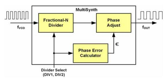
Figure 2. Silicon Labs' MultiSynth Technology
