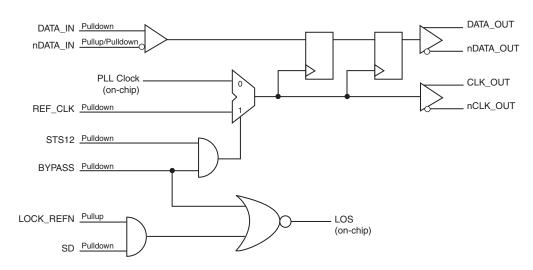
Figure 1. Signal Detect/PLL BYPASS Operation Control Diagram
