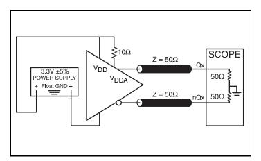
LVDS 3.3V Output Load AC Test Circuit
