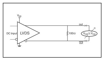
**Differential Output Voltage Setup**
