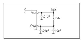
Figure 2. Power Supply Filtering
