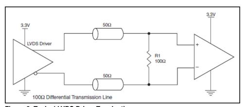
Figure 3. Typical LVDS Driver Termination
