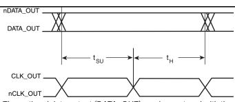
The re-timed data output (DATA\_OUT) can be captured with the rising edge of the clock output signal (CLOCK\_OUT). DATA\_OUT is valid the specified setup time before the rising CLK\_OUT signal and remains valid the specified hold time after
