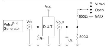
Test Circuits for All Outputs
