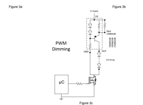
Figure 3a, 3b, 3c. Application Circuits for LED Driver with PWM Dimming Functionality
