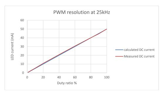
Figure 8. PWM Resolution with Power Path Switching (see Figure 3c)
