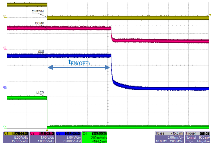
Figure 32: After EN/PWM (Yellow) goes Low for ~16 ms, the IC completely shuts down so both VDD (Blue) and COMP (Red) decay.
