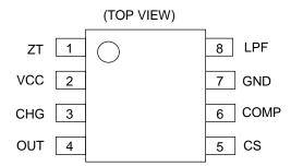
Figure 2. Pin Configuration
