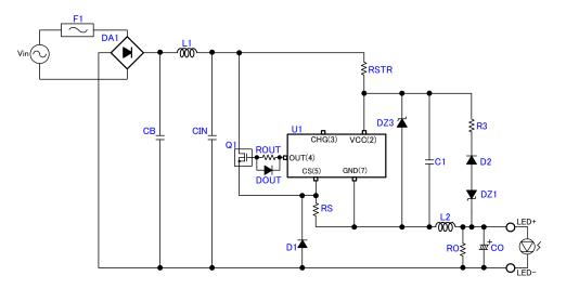
Figure 7. Application Circuit Example for DCDC (The internal charge circuit is not used)
