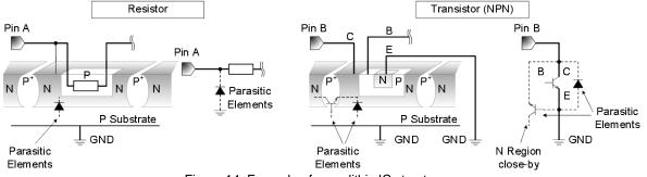
Figure 14. Example of monolithic IC structure
