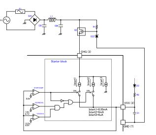
Figure 5. Charge Circuit Block Diagram
