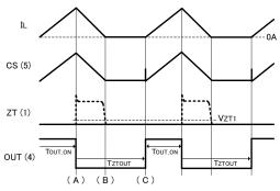
Figure 12. ZT Trigger Timeout Operation
