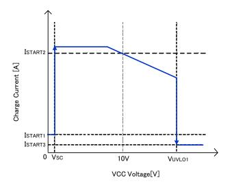
Figure 6. Charge Current-VCC Voltage Curve
