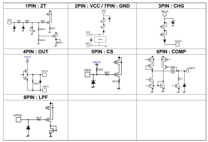
Figure 3. I/O Equivalent Circuits
