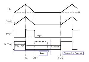
Figure 13. Maximum Frequency Operation
