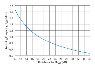
Figure 7: Typical Switching Frequency versus value of  $R_{\mathsf{FSET}}$  resistor
