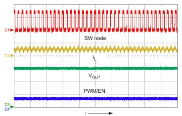
Figure 28: Normal operation of the switch node (SW); inductor current  $\,(I_L)$  and output voltage  $(V_{OUT})$  for 9 series LEDs in each of four strings configuration; shows SW node (ch1, 20 V/div.), inductor current  $I_L$  (ch2, 1 A/div.),  $V_{OUT}$  (ch3, 10 V/div.), and PWM/EN (ch4, 5 V/div.), time = 2  $\mu s/div$ .
