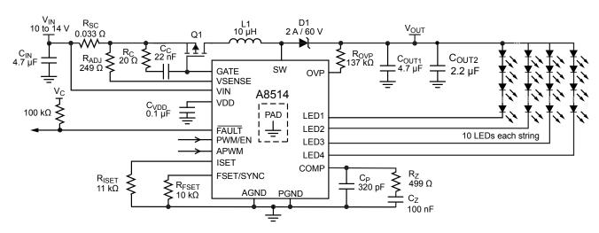
Figure 36: The schematic diagram showing calculated values from the design example above.
