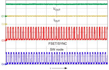
Figure 8: Diagram showing a synchronized FSET/SYNC pin and switch node; shows  $V_{OUT}$  (ch1, 20 V/div.),  $I_{OUT}$  (ch2, 200 mA/div.), FSET/SYNC (ch3, 2 V/div.), and SW node (ch4, 20 V/div.), time = 2  $\mu$ s/div.
