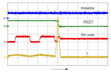
Figure 30: Secondary boost switch current limit; when this limit is hit, the A8514 immediately shuts down; shows PWM (ch1, 5 V/div.),  $V_{OUT}$  (ch2, 5 V/div.), SW node (ch3, 50 V/div.), and inductor current  $I_L$  (ch4, 2 A/div.), time = 100 ns/div.
