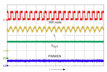
Figure 29: Cycle-by-cycle current limiting; inductor current (yellow trace,  $\rm I_L)$ , note reduction in output voltage as compared to normal operation with the same configuration (Figure 27); shows SW node (ch1, 20 V/div.), inductor current  $\rm I_L$  (ch2, 1 A/div.),  $\rm V_{OUT}$  (ch3, 10 V/div.), and PWM/EN (ch4, 5 V/div.), time = 2  $\mu s/div$ .
