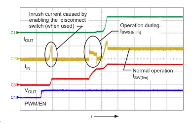
Figure 6: Startup diagram showing the input current, output voltage, and output current; shows  $I_{OUT}$  (ch1, 200 mA/div.),  $I_{IN}$  (ch2, 1 A/div.),  $V_{OUT}$  (ch3, 20 V/div.), and PWM/EN (ch4, 5 V/div.), time = 1 ms/div.
