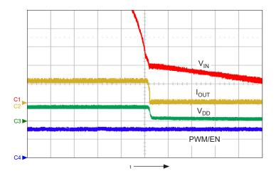
Figure 34: Shutdown showing a falling input voltage ( $V_{IN}$ ); shows  $V_{IN}$  (ch1, 2 V/div.),  $I_{OUT}$  (ch2, 200 mA/div.),  $V_{DD}$  (ch3, 5 V/div.), and PWM/EN (ch4, 2 V/div.), time = 5 ms/div.
