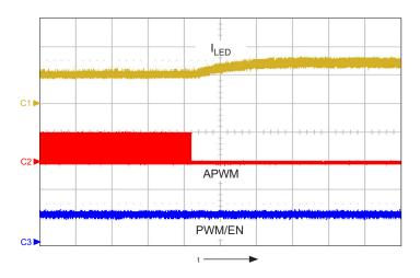
Figure 18: Diagram showing the transition of LED current from 60 mA to 80 mA, when a 25% duty cycle signal is removed from the APWM pin. PWM = 1; shows  $I_{LED}$  (ch1, 50 mA/div.), APWM (ch2, 10 V/div.), and PWM/EN (ch3, 5 V/div.), time = 500  $\mu s$ /div.
