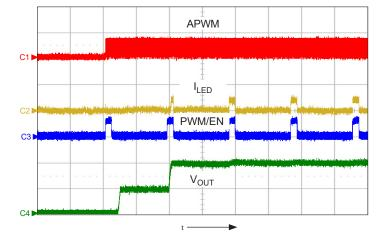
Figure 19: Diagram showing power-up sequencing LED current of 5 mA per channel with a 10% duty cycle PWM signal and a 95% duty cycle APWM signal; shows APWM (ch1, 5 V/div.),  $I_{LED}$  (ch2, 50 mA/div.), PWM/EN (ch3, 5 V/div.), and  $V_{OUT}$  (ch4, 10 V/div.), time = 500  $\mu$ s/div.
