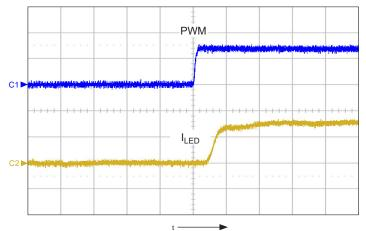
Figure 13C: Delay from rising edge of PWM signal to LED current; shows PWM (ch1, 2 V/div.), and  $I_{\rm LED}$  (ch2, 50 mA/div.), time = 200 ns/div.
