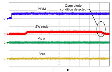
Figure 27: OVP protection when the IC is enabled during an open diode condition; shows PWM (ch1, 5 V/div.), SW node (ch2, 50 V/div.),  $V_{OUT}$  (ch3, 10 V/div.), and  $I_{OUT}$  (ch4, 200 mA/div.), time = 500  $\mu$ s/div.
