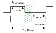
Figure 10: SYNC pulse on and off time requirements.
