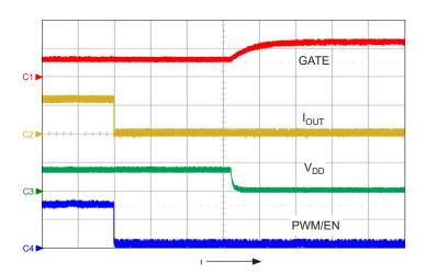
Figure 35: Shutdown using the enable function, showing the 16 ms delay between the PWM/EN signal and when the VDD and GATE of the disconnect switch turns off; shows GATE (ch1, 10 V/div.),  $I_{OUT}$  (ch2, 200 mA/div.),  $V_{DD}$  (ch3, 5 V/div.), and PWM/EN (ch4, 2 V/div.), time = 5 ms/div.
