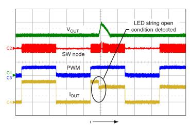
Figure 25: OVP protection in an open LED string event; shows  $V_{OUT}$  (ch1, 10 V/div.), SW node (ch2, 50 V/div.), PWM (ch3, 5 V/div.), and  $I_{OUT}$  (ch4, 200 mA/div.), time = 500  $\mu$ s/div.
