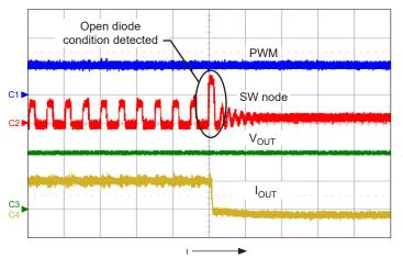
Figure 26: OVP protection in an open Schottky diode event, while the IC is in normal operation; shows PWM (ch1, 5 V/div.), SW node (ch2, 50 V/div.),  $V_{OUT}$  (ch3, 20 V/div.), and  $I_{OUT}$  (ch4, 200 mA/div.), time = 1  $\mu$ s/div.
