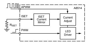
Figure 16: Simplified block diagram of the APWM and ISET circuit.
