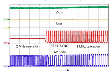
Figure 9: Transition of the SW waveform when the SYNC pulse is detected. The A8514 switching at 2 MHz, applied SYNC pulse at 1 MHz; shows  $V_{OUT}$  (ch1, 20 V/div.),  $I_{OUT}$  (ch2, 200 mA/div.), FSET/SYNC (ch3, 2 V/div.), and SW node (ch4, 20 V/div.), time = 5  $\mu s/div$ .
