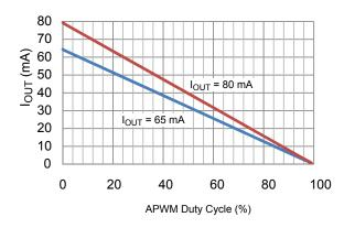
Figure 15: Output current versus duty cycle; 200 kHz APWM signal.
