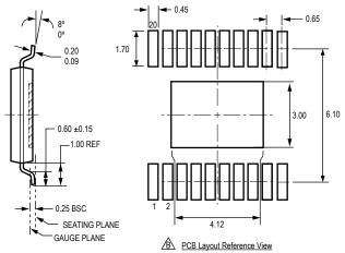
For Reference Only; not for tooling use (reference MO-153 ACT) Dimensions in millimeters
