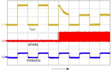
Figure 21: Transition of output current level when a 50% duty cycle signal is applied to the APWM pin, in conjunction with a 50% duty cycle PWM dimming being applied to the PWM pin; shows I<sub>OUT</sub> (ch1, 50 mA/div.), APWM (ch2, 10 V/div.), and PWM/EN (ch3, 5 V/div.), time = 500 µs/div.
