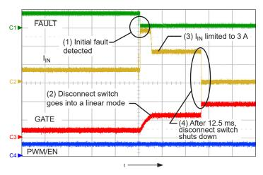
Figure 32: Showing typical wave forms for a 3-A, 1X current limit under a fault condition; shows  $f_{SW}$  = 800 kHz,  $\overline{FAULT}$  (ch1, 5 V/div.),  $I_{IN}$  (ch2, 2 A/div.), GATE (ch3, 5 V/div.), and PWM/EN (ch4, 5 V/div.), time = 5 ms/div.
