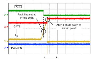
Figure 33: 2× mode, secondary overcurrent fault condition.  $I_{IN}$  is the input current through the switch. The Fault flag is set at the 1× current limit, and when the 2× current limit is reached the A8514 disables the gate of the disconnect switch (GATE); shows  $\overline{FAULT}$  (ch1, 5 V/div.), GATE (ch2, 10 V/div.),  $I_{IN}$  (ch3, 2 A/div.), and PWM/EN (ch4, 5 V/div.), time = 5  $\mu$ s/div.
