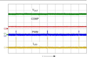
Figure 13B: Typical PWM diagram showing  $V_{OUT}$ ,  $I_{LED}$ , and COMP pin as well as the PWM signal. PWM dimming frequency is 500 Hz at 1% duty cycle ; shows  $V_{OUT}$  (ch1, 10 V/div.), COMP (ch2, 2 V/div.), PWM (ch3, 5 V/div.), and  $I_{LED}$  (ch4, 50 mA/div.), time = 500  $\mu$ s/div.
