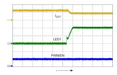
Figure 23: Example of the disabling of an LED string when the LED pin voltage is increased above 4.6 V; shows  $I_{OUT}$  (ch1, 200 mA/div.), LED1 (ch2, 5 V/div.), and PWM/EN (ch3, 5 V/div.), time = 10  $\mu$ s/div.
