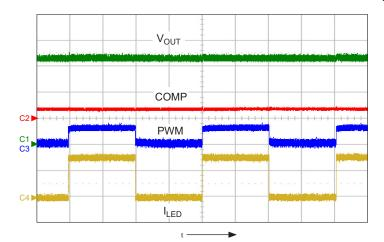
Figure 13A: Typical PWM diagram showing  $V_{OUT}$ ,  $I_{LED}$ , and COMP pin as well as the PWM signal. PWM dimming frequency is 500 Hz at 50% duty cycle; shows  $V_{OUT}$  (ch1, 10 V/div.), COMP (ch2, 2 V/div.), PWM (ch3, 5 V/div.), and  $I_{LED}$  (ch4, 50 mA/div.), time = 500  $\mu$ s/div.
