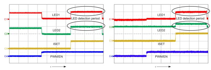
Figure 4A: An LED detect occurring when both LED pins are selected to be used; shows LED1 (ch1, 500 mV/div.), LED2 (ch2, 500 mV/div.), ISET (ch3, 1 V/div.), and PWM/EN (ch4, 5 V/div.) pins, time = 500  $\mu$ s/div.
