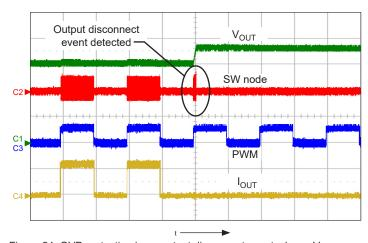
Figure 24: OVP protection in an output disconnect event; shows V $_{\rm OUT}$  (ch1, 10 V/div.), SW node (ch2, 50 V/div.), PWM (ch3, 5 V/div.), and I $_{\rm OUT}$  (ch4, 200 mA/div.), time = 1 ms/div.
