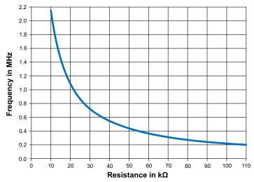
Figure 8: Switching Frequency versus R<sub>FSET</sub> Resistor
