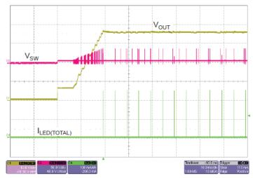
Start up at 0.02% PWM Dimming,  $V_{IN} = 7 \text{ V}$ , 4 Channels, 10 LEDs/Channel, 60 mA/Channel; Time base = 10 ms/Div
