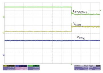
Figure 25: Disabling of LED1 String when the LED1 Pin Voltage is Increased Above 4.6 V
