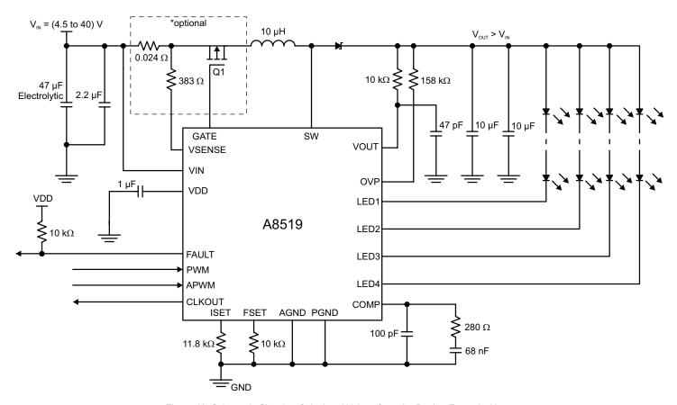
Figure 40: Schematic Showing Calculated Values from the Design Example Above
