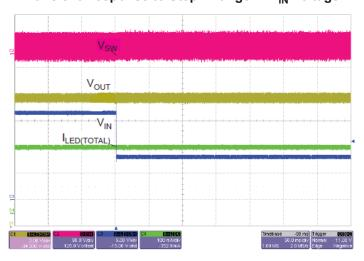
From  $V_{IN}$  = 16 V to  $V_{IN}$  = 5.5 V, 4 Channels, 60 mA/Channel, PWM = 100%; Time base = 50 ms/Div
