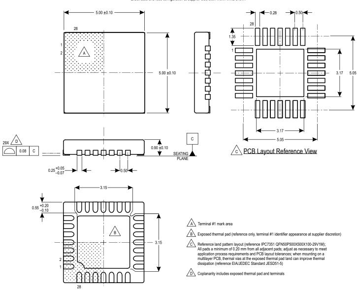
Figure 42: Package ET: 28-Pin QFN with Exposed Thermal Pad
