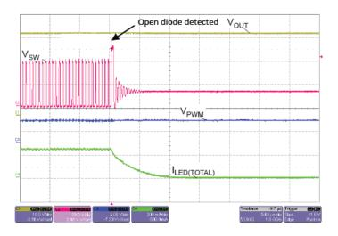
Figure 28: Open Schottky Diode Protection
