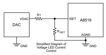
Figure 24: Typical Application Circuit Using a DAC and  $R_{\rm ISET}$  Resistor to Control the LED Current in the A8519
