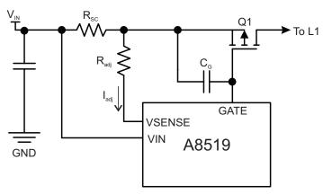
Figure 32: Typical Circuit Showing Implementation of Input
