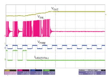
Figure 26: Output of A8519 when Disconnected from Load During Normal Operation
