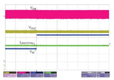
From  $V_{IN}$  = 5.5 V to  $V_{IN}$  = 16 V, 4 Channels, 60 mA/Channel, PWM = 100%; Time base = 50 ms/Div
