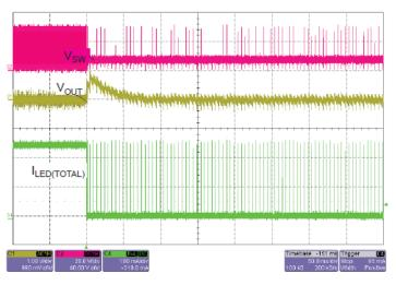
From PWM = 100% to PWM = 0.1% at 4 Channels, 60 mA/Channel,  $V_{IN}$  = 12 V; Time base = 50 ms/Div
