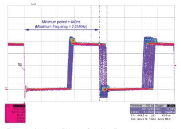
Figure 37: Maximum Dithering Switching Frequency = 2.23 MHz at  $V_{\rm IN}$  = 12 V, and PWM Ratio = 100%
