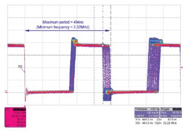
Figure 36: Minimum Dithering Switching Frequency = 2.02 MHz at  $V_{\rm IN}$  = 12 V, and PWM Ratio = 100%
