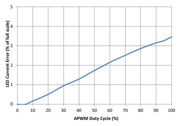
Figure 19: Error in LED Current vs. APWM Duty Cycle  $V_{IN}$  = 9 V,  $V_{OUT}$  = ~22 V,  $R_{ISET}$  = 24 k $\Omega$ , APWM = 200 kHz
