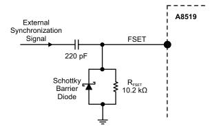
Figure 12: Countermeasure to Prevent External Sync Signal Stuck-at-Low Fault.
