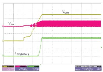
Start up at 100% PWM Dimming,  $V_{IN} = 7 \text{ V}$ , 4 Channels, 10 LEDs/Channel, 60 mA/Channel; Time base = 10 ms/Div
