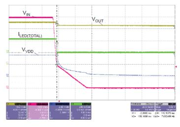
Figure 34: Shutdown with Falling Input Voltage
