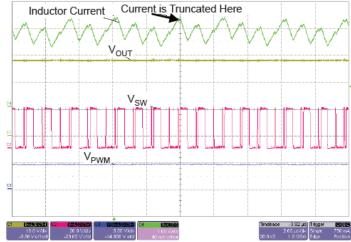
Figure 30: Cycle-by-Cycle Current Limit
