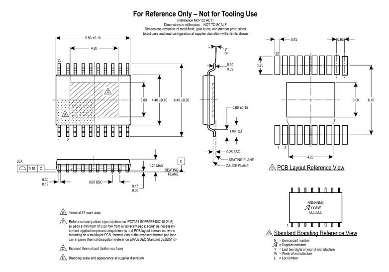
Figure 41: Package LP: 20-Pin, 0.65 mm Pin Pitch TSSOP with Exposed Thermal Pad
