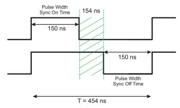
Figure 9: Sync Pulse On- and Off-Time Requirements
