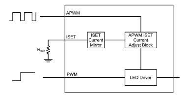
Figure 17: Simplified Block Diagram of APWM ISET Block
