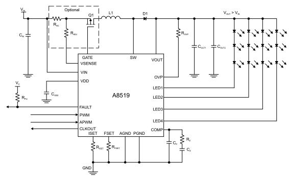
Typical Application Showing Boost Configuration with Input Disconnect Switch to Protect Against VOUT-to-Ground Short
