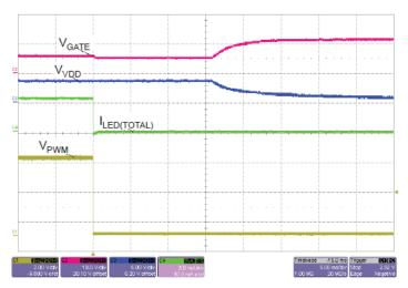
Figure 35: Shutdown Using the PWM Enable
