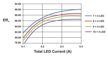
A8519 Evaluation Board Efficiency versus Total LED Current while Disconnect Switch and Snubber Circuit are Used
