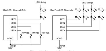
Figure 3: Channel Select Setup
