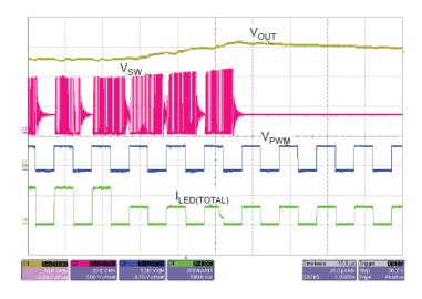
Figure 27: Typical OVP Condition Caused by an Open LED String
