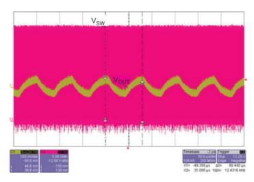
Figure 38: Output Voltage Ripple Frequency Due to Dithering = 12.4 kHz at  $\text{V}_{\text{IN}}$  = 12 V, and PWM Ratio = 100%
