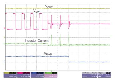
Figure 31: Secondary Boost Switch OCP
