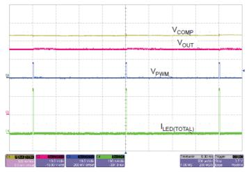
Figure 14: Typical PWM Diagram Showing V<sub>OUT</sub>, I<sub>LED</sub>, and COMP Pin, as well as the PWM Signal. (PWM dimming frequency is 500 Hz 1% duty cycle.)
