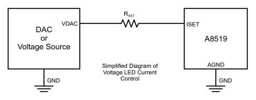
Figure 23: Typical Application Circuit Using a DAC to Control the LED Current in the A8519
