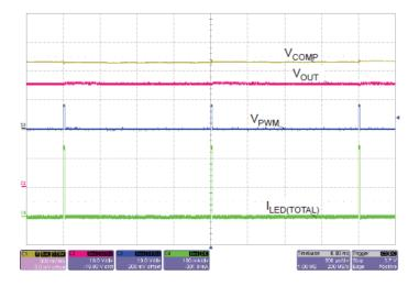
Figure 15: Rising Edge PWM Signal to Total LED Current I<sub>LED(TOTAL)</sub> Turn-On Delay; Time base = 100 ns
