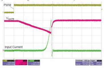
Figure 33: Startup into Output Shorted to GND fault. Input OCP tripped at 4 A ( $R_{SC}$  = 0.024 W,  $R_{adj}$  =383  $\Omega$ )
