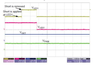
Figure 6: One LED Pin is Shorted to GND.
