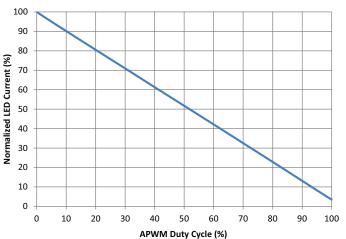
Figure 18: Normalized LED Current vs. APWM Duty Cycle  $V_{IN}$  = 9 V,  $V_{OUT}$  = ~22 V,  $R_{ISET}$  = 24 k $\Omega$ , APWM = 200 kHz
