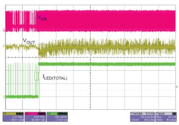
From PWM = 0.1% to PWM = 100% at 4 Channels, 60 mA/Channel,  $V_{IN}$  = 12 V; Time base = 50 ms/Div
