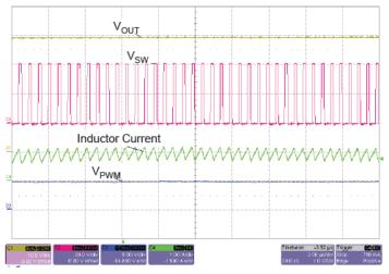
Figure 29: Normal Operation of Switch Node (V<sub>SW</sub>), Inductor Current, and Output Voltage (V<sub>OUT</sub>)
