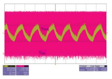
Figure 39: Output Voltage Ripple Amplitude Due to Dithering = 100 mV at  $V_{IN} = 12 \text{ V}$ , and PWM Ratio = 100%
