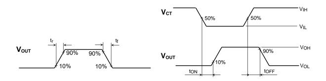
Figure 2 t<sub>r</sub>, t<sub>f</sub>, t<sub>ON</sub>, t<sub>OFF</sub> Waveforms(Active Low)
