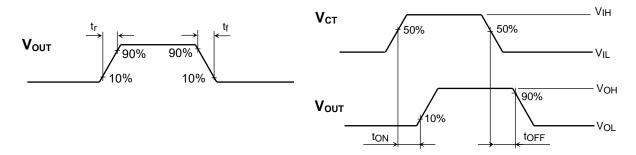
Figure 1 t<sub>r</sub>, t<sub>f</sub>, t<sub>ON</sub>, t<sub>OFF</sub> Waveforms(Active High)
