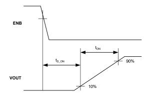
Figure 1. Turn-on Delay and Turn-on Time
