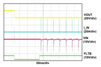
Figure 11. Short Circuit Response (C<sub>SS</sub> = 1nF, No Load, Option -01)
