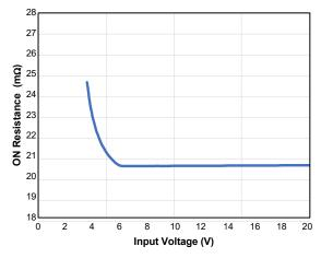
Figure 20. On Resistance vs. Input Voltage
