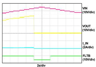
Figure 10. Over Voltage Protection (Option -02)
