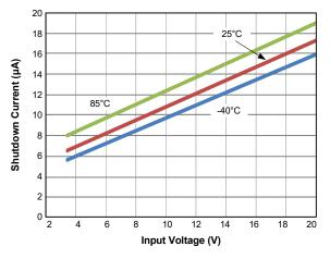
Figure 16. Shutdown Current vs. Input Voltage
