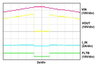
Figure 9. Over Voltage Protection (Option -01)
