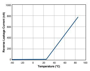
Figure 17. Reverse Leakage Current vs. Temperature
