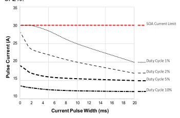
Figure 23. Pulsed current magnitude vs duration for a given duty cycle
