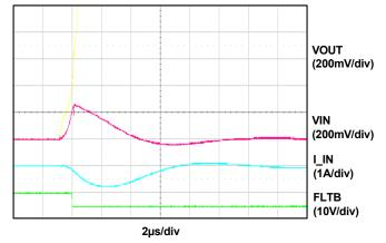
Figure 7. Shutdown (VIN = 5V)
