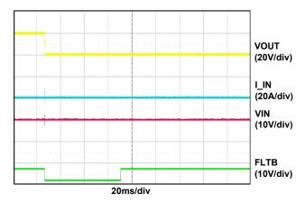
Figure 12. Short Circuit Response (C<sub>SS</sub> = 1nF, No Load, Option -02)
