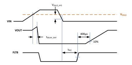
Figure 2. OVP Delay and Recovery Time (AOZ1327DI-01)
