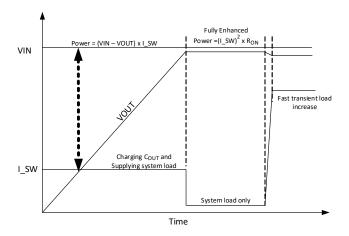
Figure 21. Soft start power dissipation
