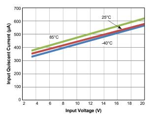
Figure 15. Quiescent Current vs. Input Voltage
