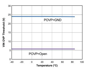
Figure 18. VIN OVP vs. Temperature
