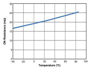
Figure 19. On Resistance vs. Temperature
