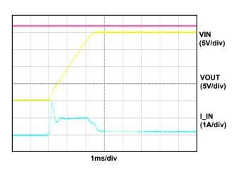
Figure 5. Soft Start Ramp (VIN = 5V)
