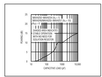
Figure 7. Peaking vs. Capacitive Load
