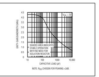
Figure 8. MAX4250–MAX4254 Unity-Gain Bandwidth vs. Capacitive Load
