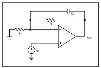
Figure 1. Adding Feed-Forward Compensation
