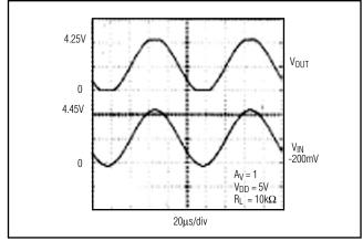
Figure 4. Rail-to-Rail Output Operation
