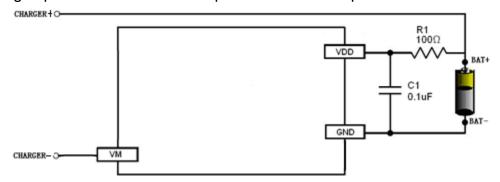
Fig 6 XB3306D in a Typical Battery Protection Circuit
