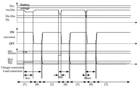
Figure 5-2 Overdischarge Current Detection
