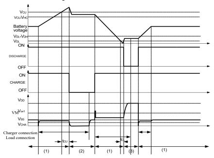
Figure 5-1 Overcharge and Overdischarge Voltage Detection
