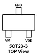
Figure 2. PIN Configuration
