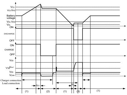
Figure 5-1 Overcharge and Overdischarge Voltage Detection
