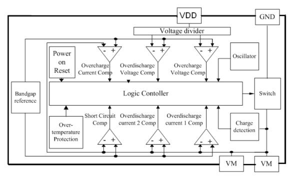
Figure 3. Functional Block Diagram
