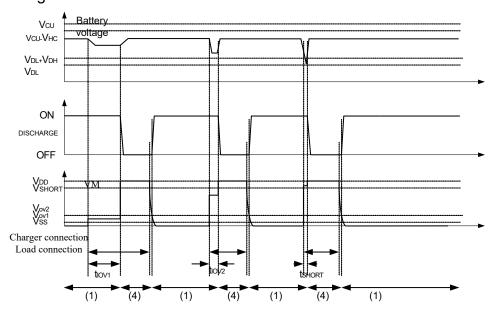
**Figure5-2 Overdischarge Current Detection**
