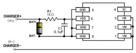
Fig 6 XB8608AJ in a Typical Battery Protection Circuit
