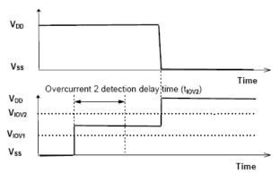
Figure 4. Overcurrent delay time
