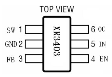
Figure 3. PIN Configuration
