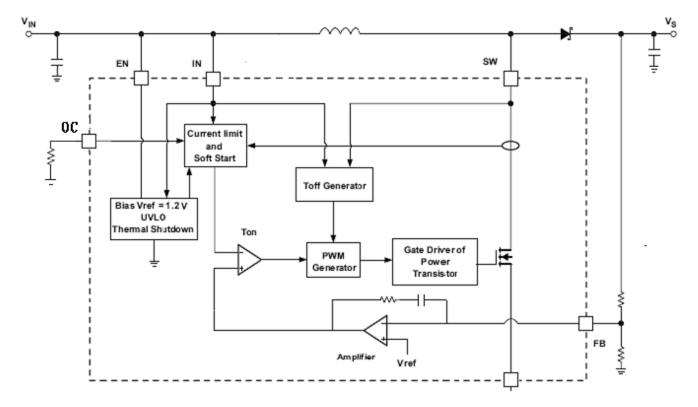
Figure 4. Functional Block Diagram
