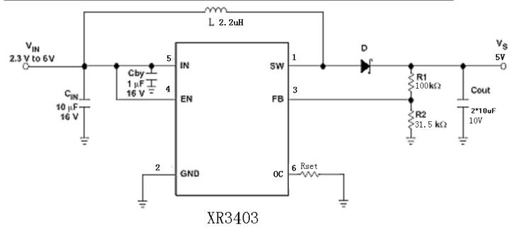
Figure 2. Typical Application Circuit2
