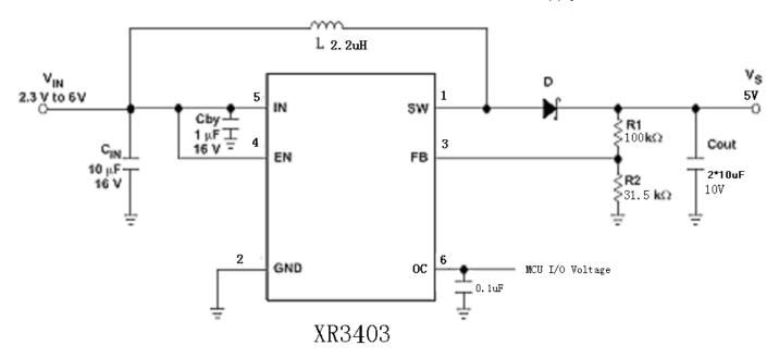
Figure 1. Typical Application Circuit1
