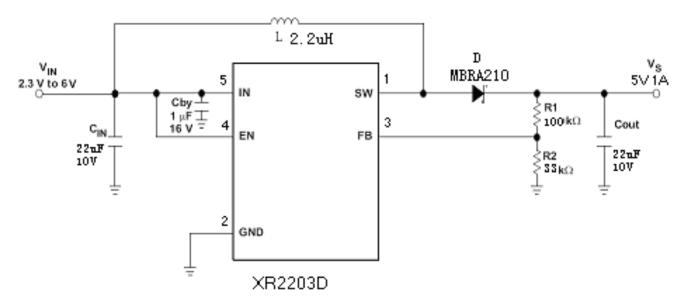
Figure 1. Typical Application Circuit1
