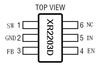
Figure 2 PIN Configuration
