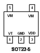
Figure 2. PIN Configuration
