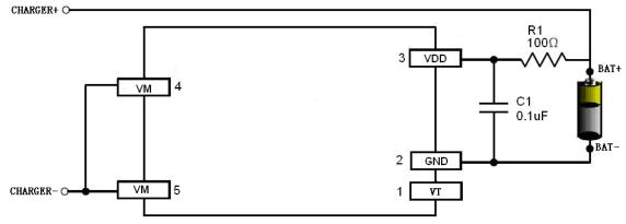
Fig 6 XB5556A0 in a Typical Battery Protection Circuit
