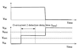
Figure 4. Overcurrent delay time
