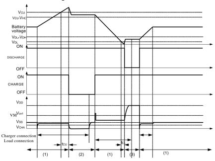
Figure 5-1 Overcharge and Overdischarge Voltage Detection
