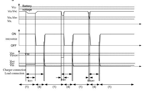
**Figure5-2 Overdischarge Current Detection**
