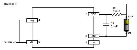
Figure 1. Typical Application Circuit
