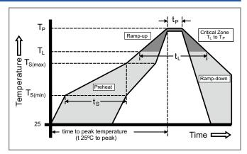
Soldering Parameters - Wave Soldering (Thru-Hole Devices)
