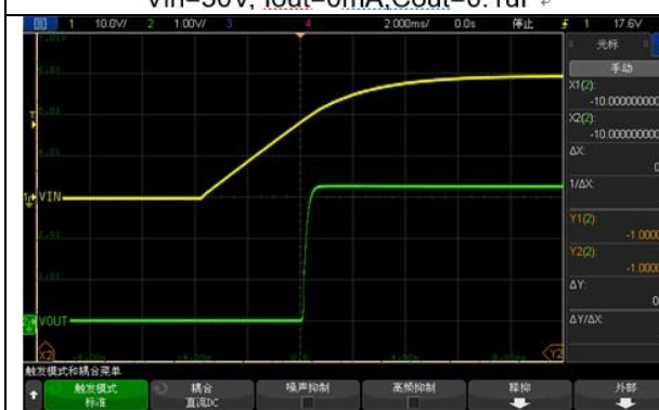
Vin=30V, Iout=30mA, Cout=0.1uF
