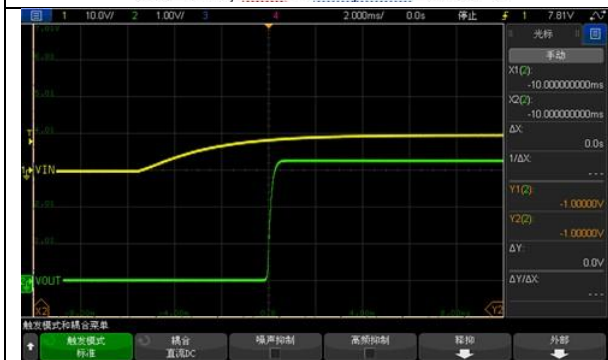
Vin=10V, Iout=30mA, Cout=0.1uF
