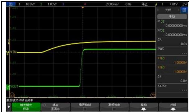
Vin=10V, Iout=0mA, Cout=0.1uF
