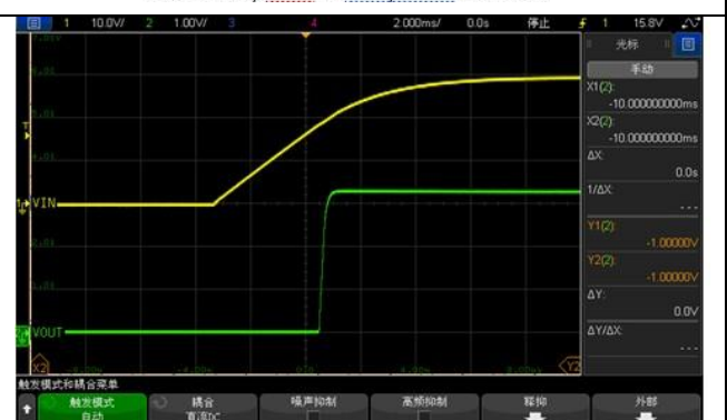
Vin=30V, Iout=30mA, Cout=10uF
