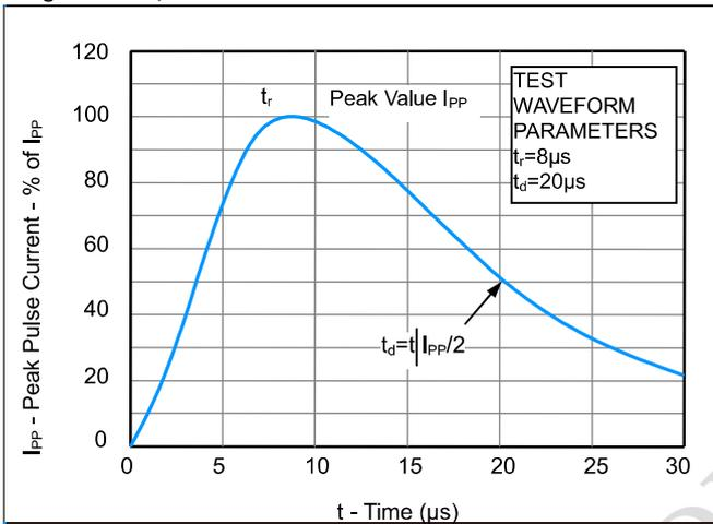
Fig2. ESD Pulse Waveform (according to IEC 61000-4-2)
