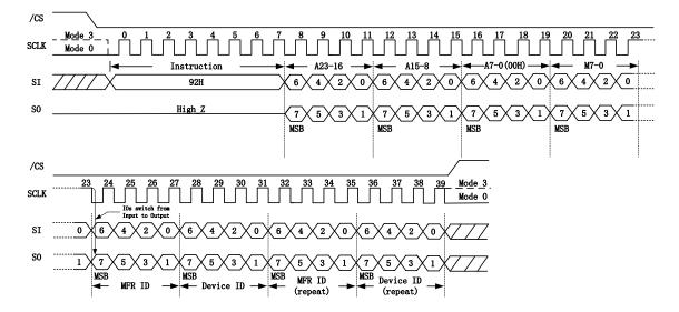
Figure 7.3.4. Read Manufacturer / Device ID Dual I/O Instruction
