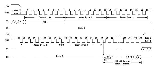
Figure 7.3.7. Read Unique ID Sequence Diagram
