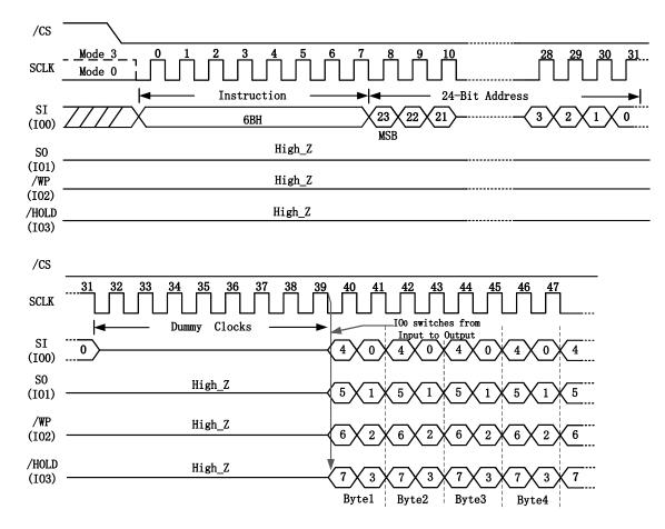
Figure 7.2.4. Fast Read Quad Output Instruction
