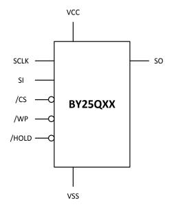
Figure 2. Pin Configuration SOP8/TSSOP8
