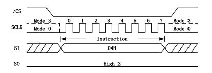
Figure 7.1.3. Write Disable Instruction for SPI Mode
