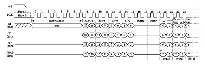
**Figure 7.2.6a.** Fast Read Quad I/O Instruction (Initial instruction or previous M5-4≠10)
