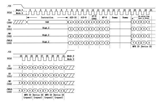
Figure 7.3.5. Read Manufacturer / Device ID Quad I/O Instruction
