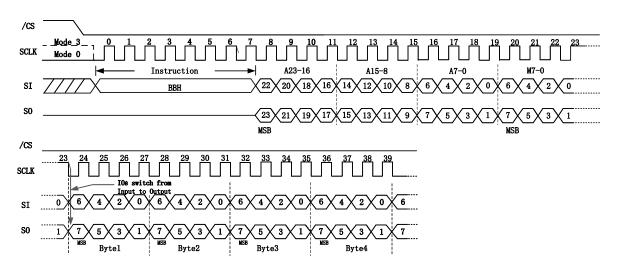
Figure 7.2.5a. Fast Read Dual I/O Instruction (Initial instruction or previous M5-4 \ne 10)
